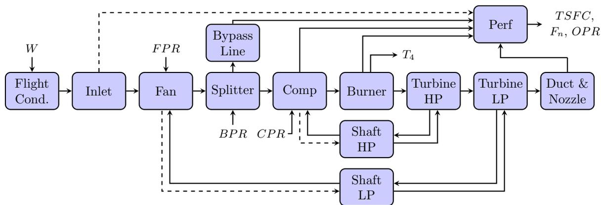
Figure 21. Optimal model coupling for  $\lambda = 1.0 \times 10^{-1}$
