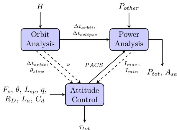
Figure 9. Optimal model coupling for  $\lambda = 1.0 \times 10^{-3}$
