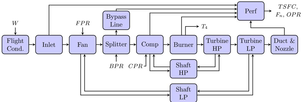
Figure 19. Turbine engine cycle model from Ref. 38
