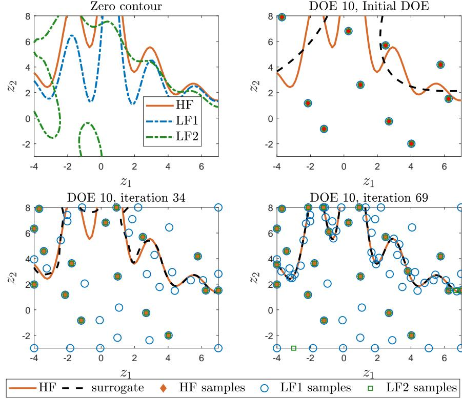
Figure 7: Progress of mfEGRA at several iterations showing the surrogate prediction and the samples from different models for a particular initial DOE. HF refers to high-fidelity model  $g_0$ , LF1 refers to low-fidelity model  $g_1$ , and LF2 refers to low-fidelity model  $g_2$ .
