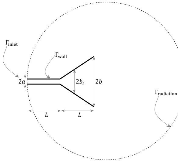
Figure 8: Two-dimensional acoustic horn geometry with  $a = 0.5, b = 3, L = 5$  and shape of the horn flare described by six equally-spaced half-widths  $b_1 = 0.8, b_2 = 1.2, b_3 = 1.6, b_4 = 2, b_5 = 2.3, b_6 = 2.65$ . [37]
