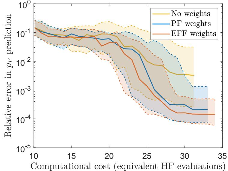
Figure 4: Effect of different weights for information gain criterion in mfEGRA for analytic test problem in terms of convergence of relative error in  $p_F$  prediction (shown in log-scale) for 100 different initial DOEs. Solid lines represent the median and dashed lines represent the 25 and 75 percentiles.
