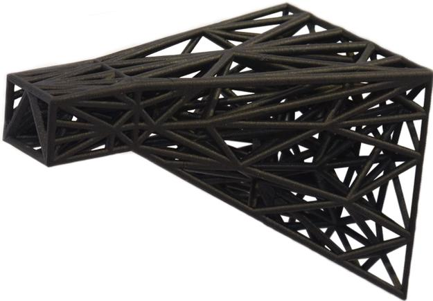
Fig. 21: This heterogeneous cellular structure is manufactured using the Markforged Mark II desktop printer.
