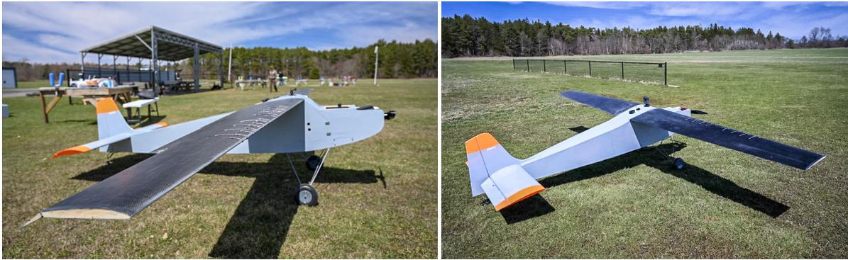
**Fig. 4** The custom-built hardware testbed used in this research. We create a digital twin of this 12-foot wingspan aircraft, and update the digital twin in response to online data from structural sensors on the aircraft wings.
