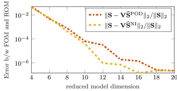
Figure 7: Tubular reactor example: Relative state errors produced by both ROMs, i.e.,  $\|\mathbf{S} - \mathbf{V}\widehat{\mathbf{S}}^{\text{POD}}\|_2 / \|\mathbf{S}\|_2$  and  $\|\mathbf{S} - \mathbf{V}\widehat{\mathbf{S}}^{\text{NI}}\|_2 / \|\mathbf{S}\|_2$ .
