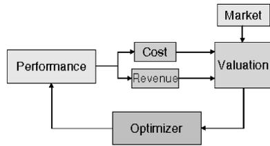
Fig. 1 Block diagram depiction of value-based MDO framework.
