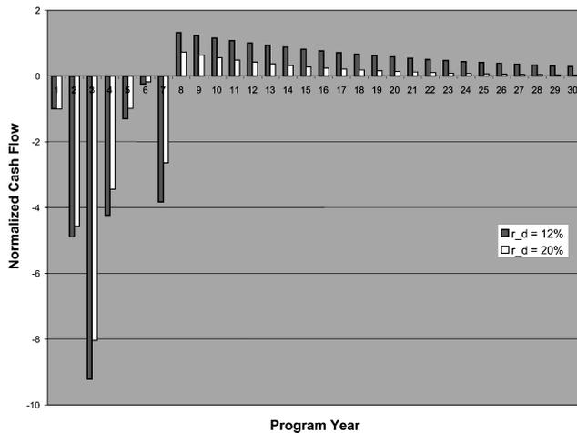
**Fig. 2** Series of cash flows for program designs optimized using deterministic NPV at discount rates of 12% and 20%. Heavier discounting causes later profits to affect NPV less, causing the initial costs incurred to drive the value optimization. Values are normalized by the cash flow in year 1.
