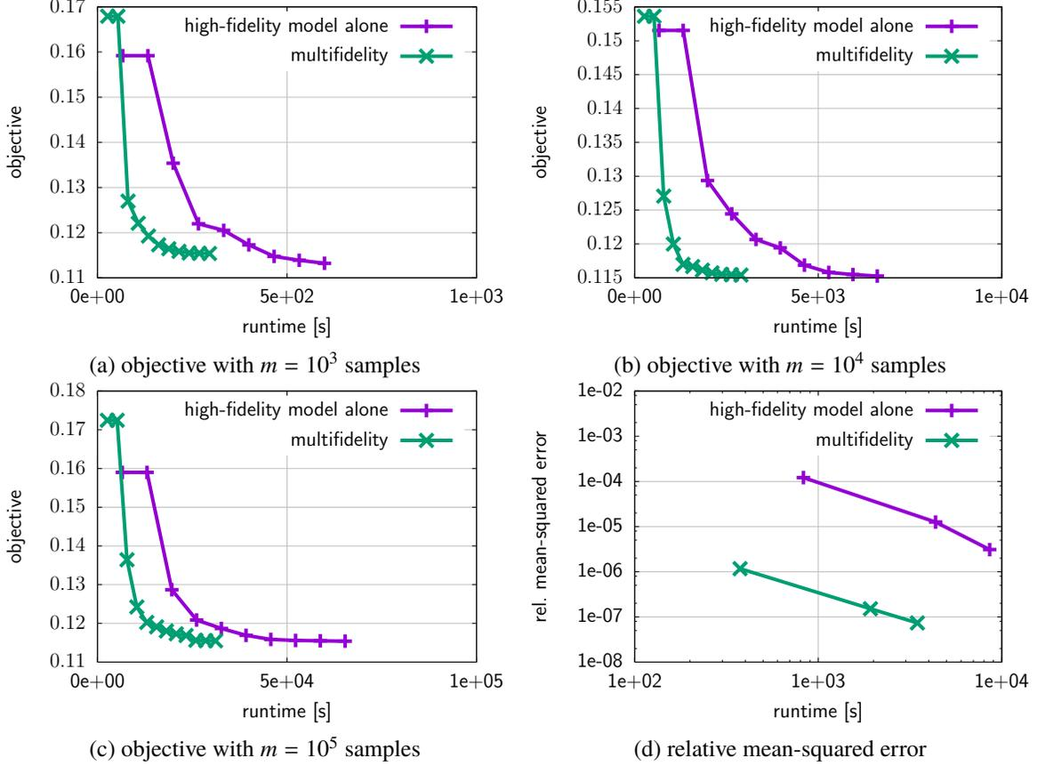
Fig. 4 Heat example: The probability level is set to  $\beta = 10^{-7}$ . Plots (a)-(c) show the value of the objective function for the single-fidelity and the multifidelity approach. The costs of the multifidelity approach seem lower than the costs of the single-fidelity approach that uses the high-fidelity model alone. The relative mean-squared error plotted in (d) shows that the multifidelity approach achieves a speedup of up to two orders of magnitude in this example.
