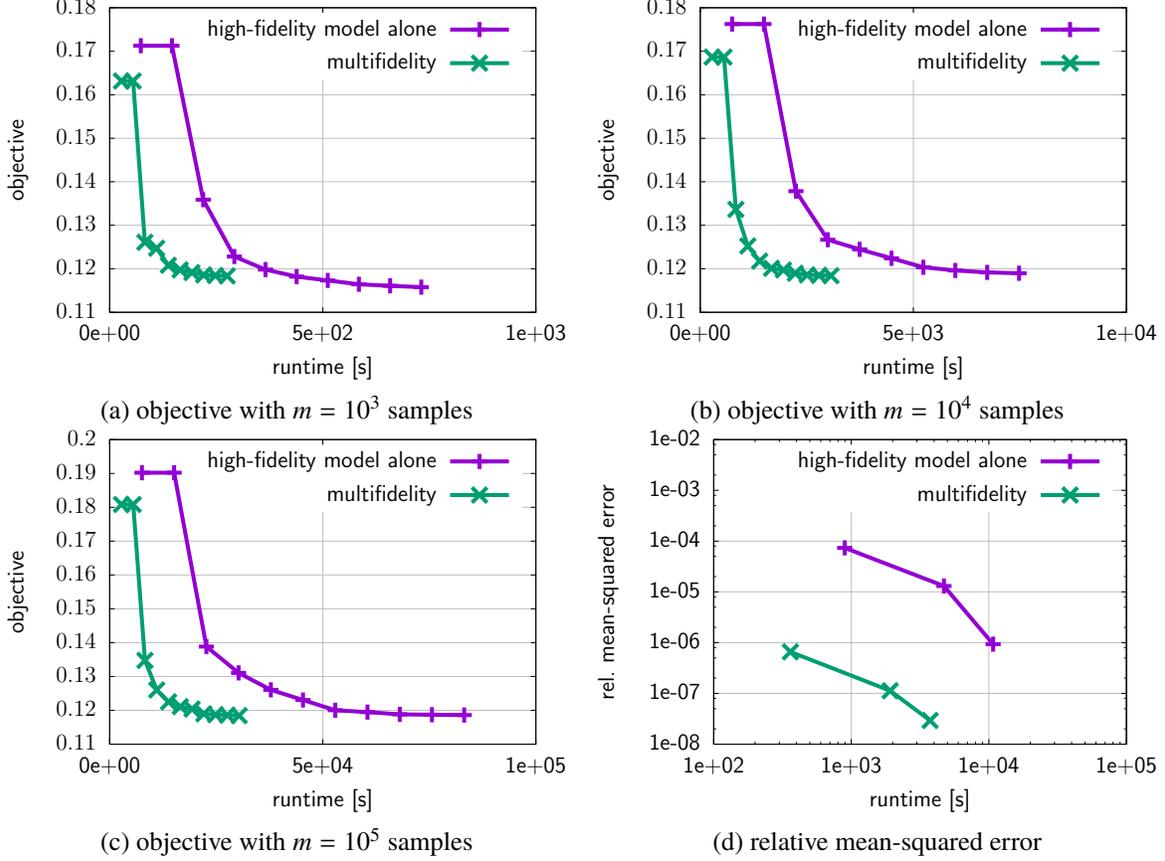
Fig. 5 Heat example: The probability level is set to  $\beta = 10^{-8}$ . The plots (a)-(c) show the convergence history of the multifidelity and the single-fidelity approach. A speedup of up to two orders of magnitude is obtained with the multifidelity approach with respect to the relative mean-squared error in the objective value compared to the single-fidelity approach, see plot (d).
