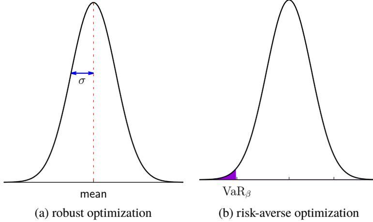
Fig. 2 Robust optimization penalizes deviations from the mean behavior, indicated by the standard deviation  $\sigma$  in plot (a). In contrast, risk-averse optimization emphasizes rare and low-probability events that are in the tails of the distribution, see plot (b). The  $\text{VaR}_\beta$  is the  $\beta$ -quantile of the distribution and  $\text{CVaR}_\beta$  is the expectation in the tail conditioned on the  $\text{VaR}_\beta$ , which is indicated by the shaded area in (b).
