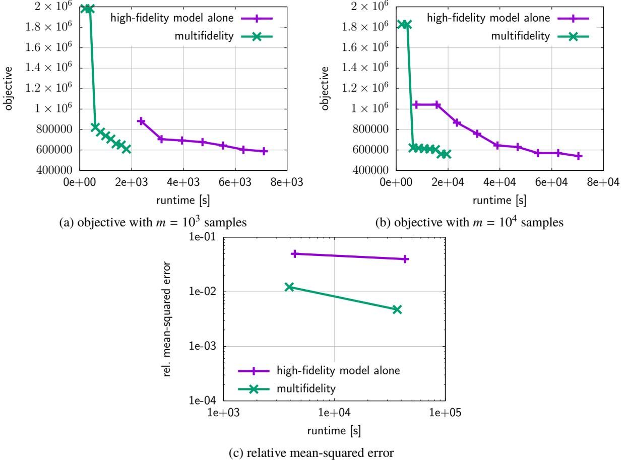
Fig. 8 Coupled aero-structural optimization: The plots in (a) and (b) show the objective value versus the costs for probability level  $\beta = 10^{-6}$ . Note that in plot (a) the value of the objective corresponding to the single-fidelity approach with the high-fidelity model alone is approximately  $10^{12}$  in the first two iterations and therefore truncated from the plot. Plot (c) shows the runtime of the multifidelity risk-averse optimization versus the relative mean-squared error.
