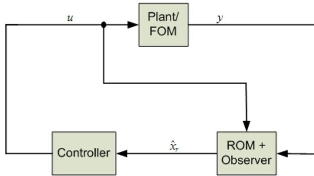
**Figure 1. Block diagram of the output-feedback setup. In this case  $\hat{x}_r$  is an estimate of the reduced state  $x_r$  based on an observer using the reduced model (ROM) and measurements from the CFD model (FOM).**
