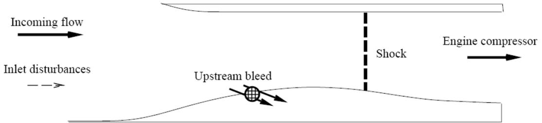
Figure 2. Active flow control setup for the supersonic inlet.<sup>38</sup>
