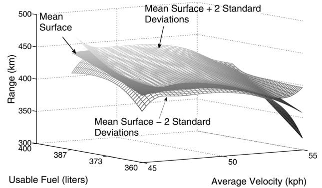
**Fig. 4** Gaussian process model of a candidate IFV design. The lighter gray surfaces represent the  $\pm 2$  standard deviation surfaces from the mean surface, which is shown as the darker mesh between the top and bottom surfaces.
