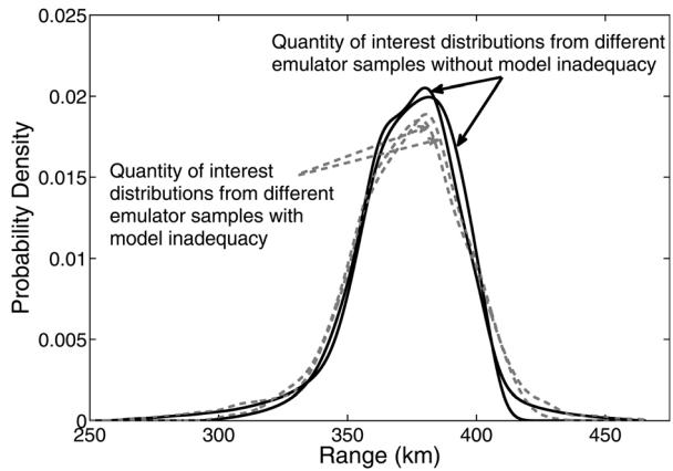
**Fig. 5** Probability density functions of the range of the IFV. The solid lines represent two distributions that were estimated using two different samples of the Gaussian process emulator. The dashed gray lines are the output distributions from the same two samples of the Gaussian process emulator; however, for these distributions, model inadequacy has been included.
