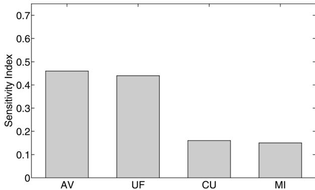
**Fig. 6** Sensitivity indices of the four factors that impact the complexity of the IFV design with respect to range. From left to right the indices are for average velocity (AV), usable fuel (UF), code uncertainty (CU), and model inadequacy (MI).
