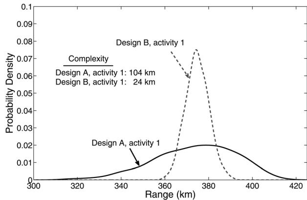
**Fig. 7** Sampled distributions and complexity estimates of the range quantity of interest of the two different IFV design options. Design A uses newer technology for the vehicle velocity control and fuel systems, whereas design B uses older technology for both systems.
