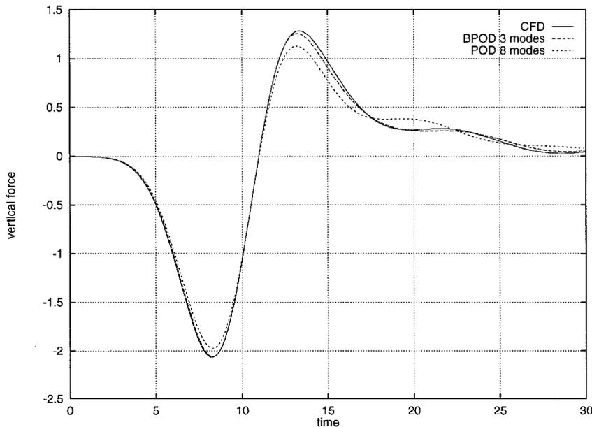
Fig. 5 Response of NACA 0012 airfoil to a pulse input in plunge:  $M = 0.755$ ,  $\alpha = 0.016$  deg, and  $g = 0.1$ . Results from CFD model (13,928 states, —), conventional POD reduced-order model (eight states, - - -), and balanced reduced-order model (three states, - - -).
