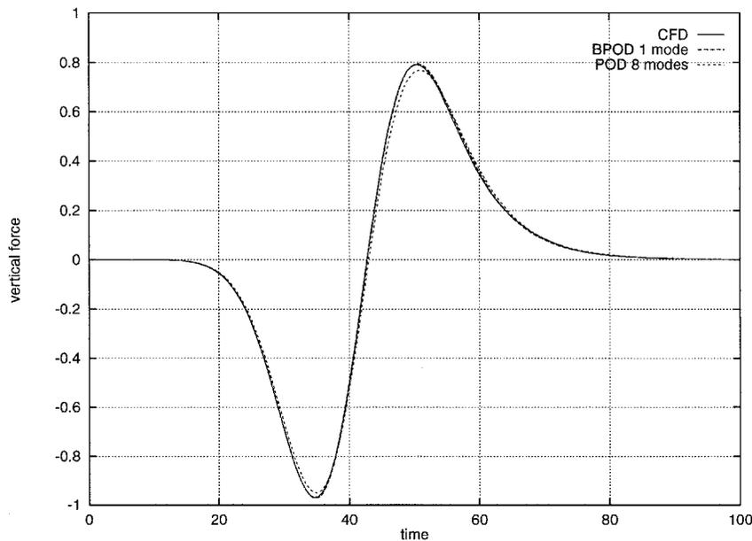
Fig. 4 Response of NACA 0012 airfoil to a pulse input in plunge:  $M = 0.755$ ,  $\alpha = 0.016$  deg, and  $g = 0.01$ ; results from CFD model (13,928 states, —), conventional POD reduced-order model with eight states (- - -), and balanced reduced-order model with one state (- - -).
